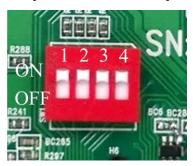
The DIP switch has four PINs, where each PIN has the two states ON and OFF. The switch can therefore represent 16 distinct station numbers, as shown in the table below. Be especially aware of the relationship between station numbers and controller parameters.
