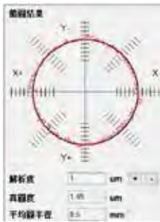
Reversal spike without compensation : 2um
